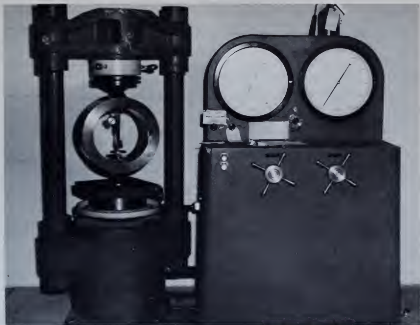
Figure 229.—Testing machine with proving ring in place prior to calibration of the machine. P382-706-11158.
